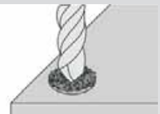
Pre-drill with spiral drill bit
