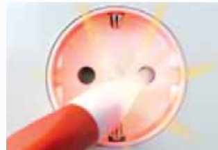
The testing pen detects the phase and neutral conductor
