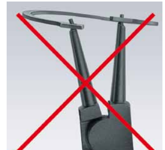
Conventional Circlip Pliers: distortion of the circlip when being fitted is possible
